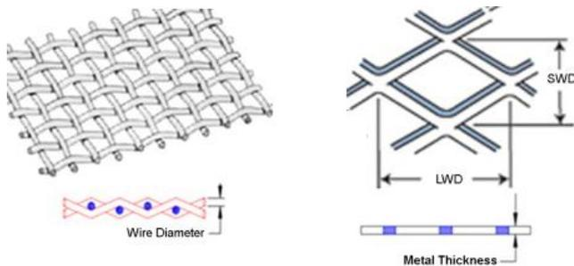
Fig. 5. Metal mesh types: woven (typical thickness is 3 times diameter of wire) and expanded (less than non expanded thickness and have better molding properties on curved surfaces)
