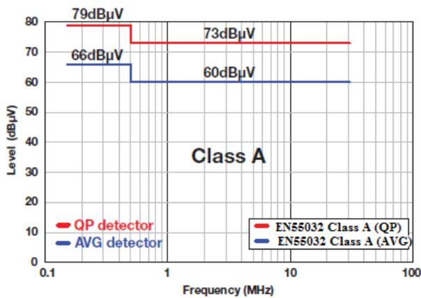
Fig. 3. European Norm EN 61000-6-4 (EN55032) – conducted emissions, mains port
