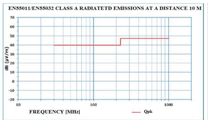
Fig. 2. European Norm EN 61000-6-4 (EN 55011, 55032) – radiated emissions
