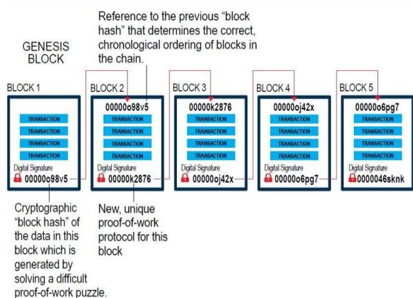
Fig. 1. Blockchain Structure source: Distributed Ledger Technology (DLT) and Blockchain FinTech Note1/ World Bank Group
